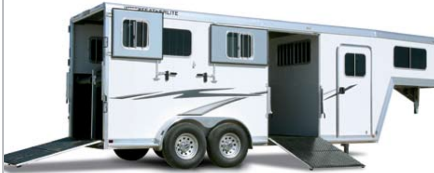
Model 9608. Specially designed for thoroughbreds, Big Horse Model 9608 features two side loading doors and rear ramp with many dressing room size choices. Available with or without side ramp.
