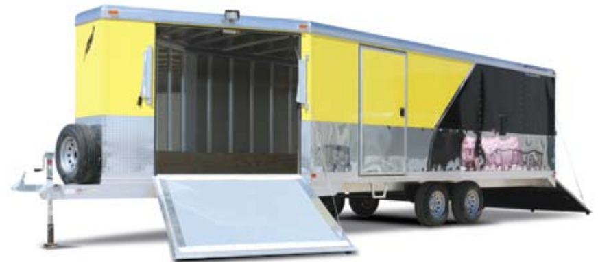
Model 1648 Snowmobile. Snowmobile trailer Model 1648 comes with a 7' v-nose. Trailer shown with optional dual color side sheets, stainless steel wrap up 24", gravel guard, spare tire, load light and cabinets.
